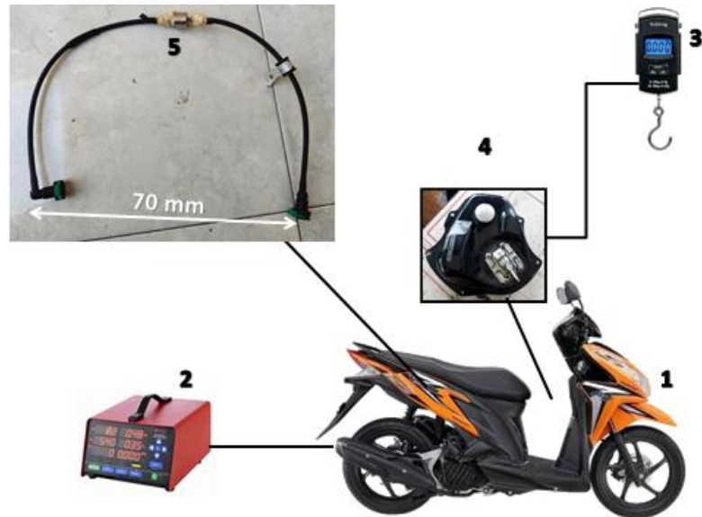
Figure 1. Testing equipment schematic. 1. Motorcycle, 2. Exhaust gas analyzer, 3. Digital-spring scale, 4. Fuel tank, 5. Fuel line with magnet
